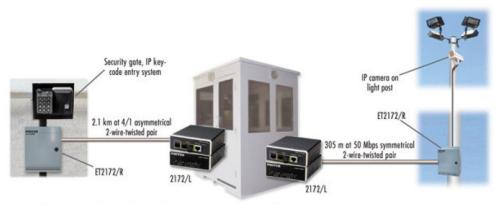
The Patton EnviroNET Ethernet Extender offers a reliable and robust solutions for connecting peered 10/100Base-T Ethernet LANs; reaching remote PCs and equipment; or delivering last-mile ISP services—at line rates up to 50 Mbps! Patton's EnviroNET allows the Ethernet Extenders to operate under harsh temperatures (-40 to 85 ℃) and resist various environmental
